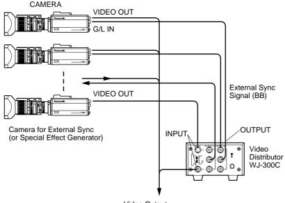
Video Output To Special Effect Generator or Monitoring System
